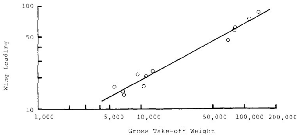
Fig. 6. Relationship between wing loading and size of aircraft, 1928–1957.
